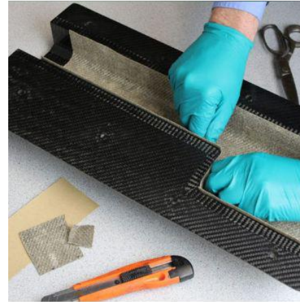
Laying up prepreg in a mould
